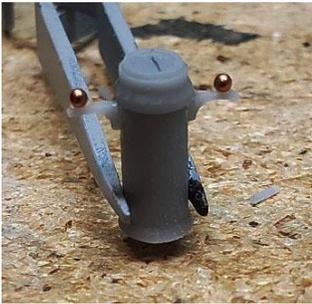
Glue the compass ball mounts on the compass 180 degrees apart. After glue has set, place a dab of canopy glue on them, and wait for it to get tacky. Once tacky, place one of the copper balls on them. After the canopy glue has set, put a touch of CA on them.
